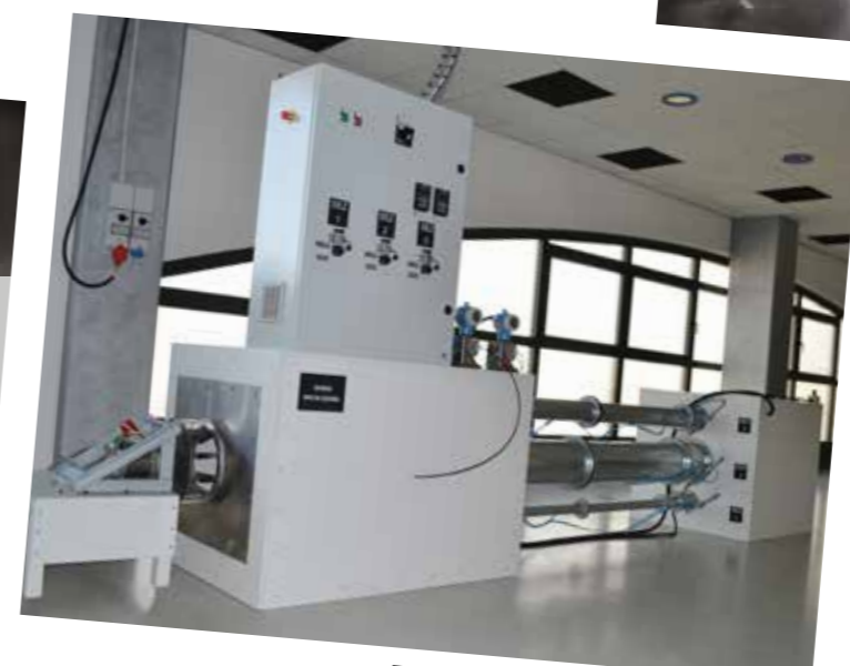
Testing Machine in compliance with ISO 5801 Norm
